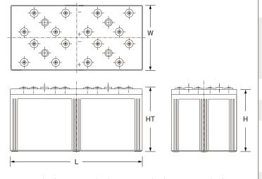
27.91 (709) **W**: 13.77 (350) **H**: 13.26 (337) **HT**: 13.74 (349) Tolerances are +/- 0.04 in. (+/- 1mm) and +/- 0.08 in. (+/- 2mm) for height dimensions. All data subject to change without notice.
